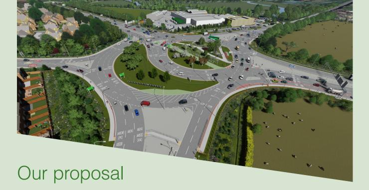
We are proposing to improve the existing roundabout at Chowns Mill, which will include widening the A45 and A6 approaches to provide additional traffic lanes, creating an additional roundabout section on the south side of the existing roundabout, and introducing traffic signals to manage traffic safely and effectively:
