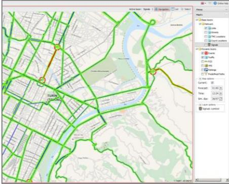
PTV Optima allows traffic managers to monitor real-time traffic and provides an overview of all existing traffic events.
