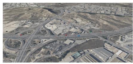
The A-70 has been designed with a new collector-distributor road in each traffic direction. These roads are conveniently connected to the trunk of the dual carriageway on the south side and to the A-77 node on the north side. This achieves a level of service between B and D in all the basic segments.
